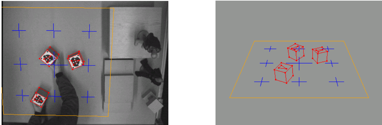
Figure 5 Three tracked cubes labeled with different coded markers (left) and generated virtual front view (right). Overlays indicate the estimated pose (red) and the calibrated world coordinate system on the stage (yellow and blue).
